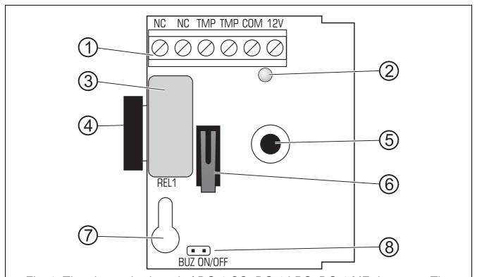
Fig. 1. The electronics board of DG-1 CO, DG-1 LPG, DG-1 ME detectors. The electronics board of DG-1 TCM detector differs in size and shape of the gas sensor installed.
